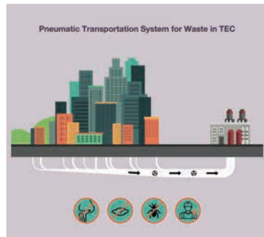
Figure 9-4: Schematic Diagram of Pneumatic Transportation System for Waste in TEC
