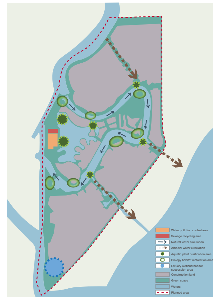
Figure 7-6: Water System Planning of the Eco-city
