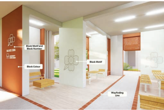
▲ Example of a BTO project designed with dementia-friendly wayfinding features, such as individualised colours and motifs to identify different blocks, and a clear wayfinding line to demarcate the main circulation route through the space.
