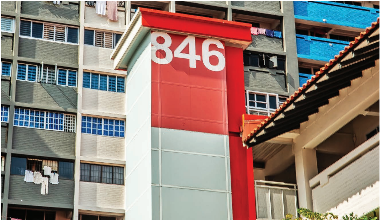
▲ HDB flats at Khatib Central are labelled clearly with distinctive block numbers located at eye level as well as at the top of the blocks, enabling people to identify the buildings from both near and far.
