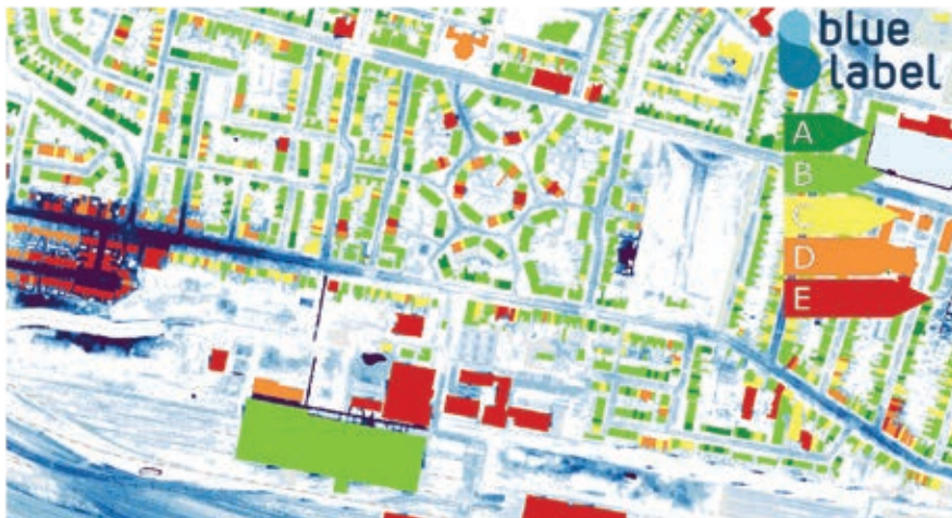
Blue Label flood risk map used to highlight infrastructure (buildings and roads) at risk of flooding from rainwater. A=smallest risk, E=highest risk.
