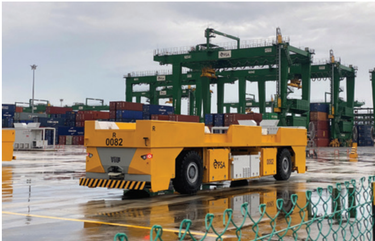
Automated guided vehicles are capable of moving cargo efficiently and securely while being greener and more sustainable compared to diesel prime movers. Image: PSA Singapore
