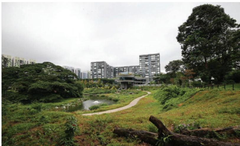
Alkaff Lake in Bidadari Park retains stormwater to prevent flooding. The accumulated stormwater is slowly discharged to Marina Reservoir. Image: NParks
