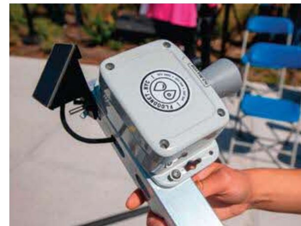
FloodNet sensors. Image: NYC DEP
