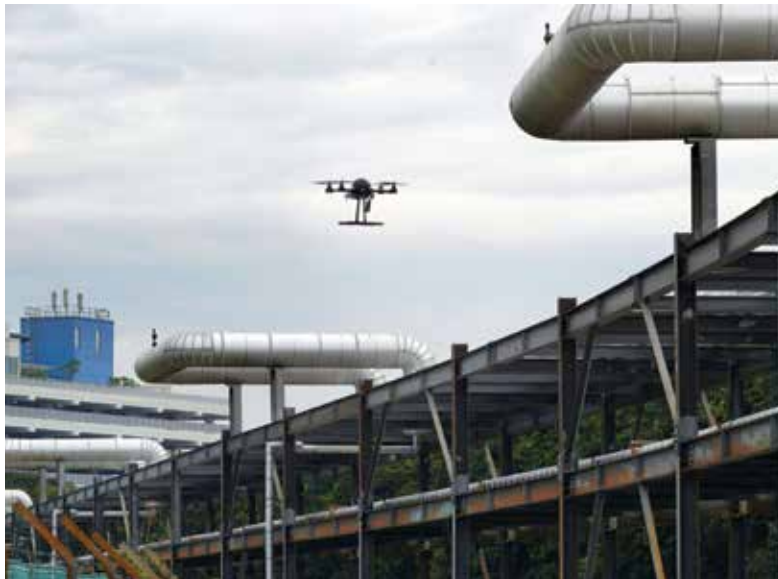
20. Demonstration of a drone inspecting chemical and utilities pipelines for leaks on Jurong Island. The drones will be equipped with multiple video cameras and sensors.
