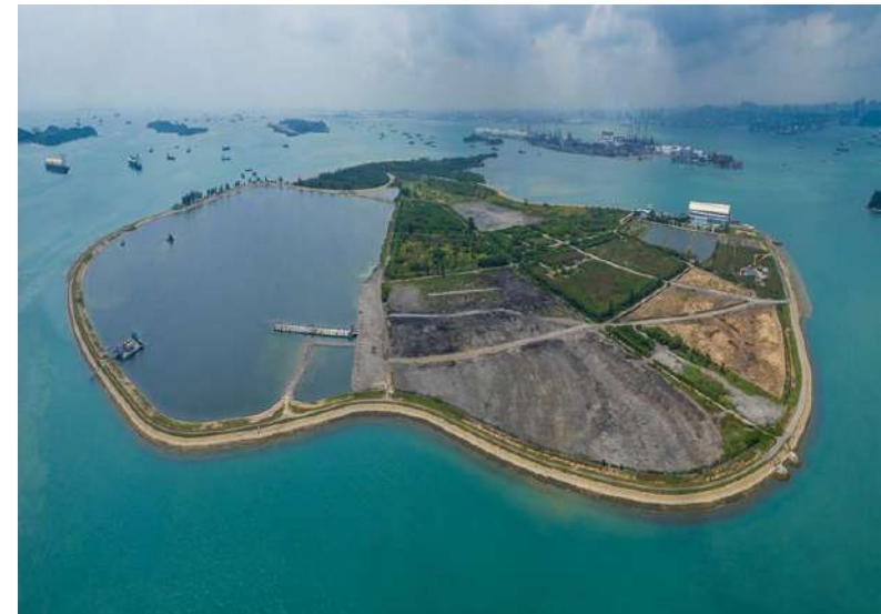
16. Incineration ash is buried at purpose-built lagoons in Semakau Landfill. Adjacent wetlands and reefs serve as bioindicators of pollution.
