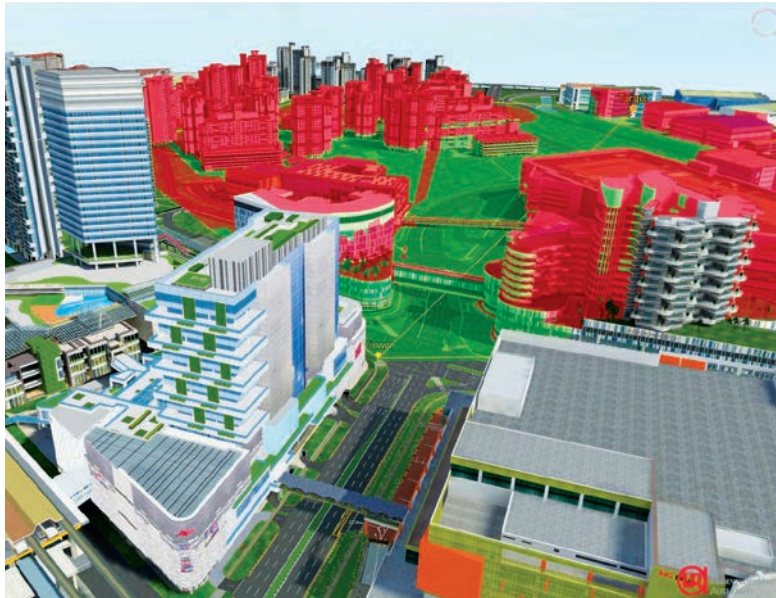
Viewshed analysis using the URA's 3D Urban Model to analyse viewable area from an onlooker perspective at Jurong Gateway Area.
