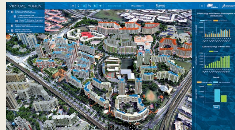
Analysis of potential for solar energy production using Virtual Singapore. Image courtesy of National Research Foundation Singapore, Singapore Land Authority, Government Technology Agency of Singapore, and Dassault Systèmes.
